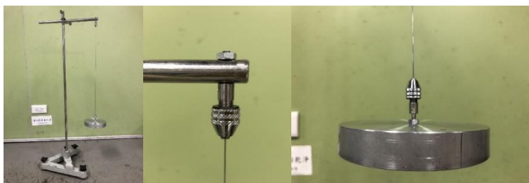
Fig. 10: Experimental setup of torsion pendulum with a hanging calibration object.
